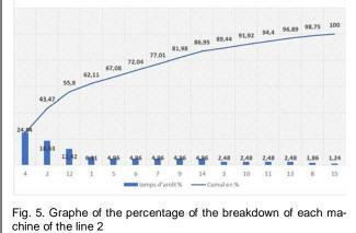
According to the Pareto chart, we see that 81.98% of shutdown problems of line 2 are due to shutdowns of machines: 4, 2, 12, 1, 5, 6, 7 and 9. These breakdown periods take up a significant part of working time and therefore contribute to the slowing and/or stopping of production.
